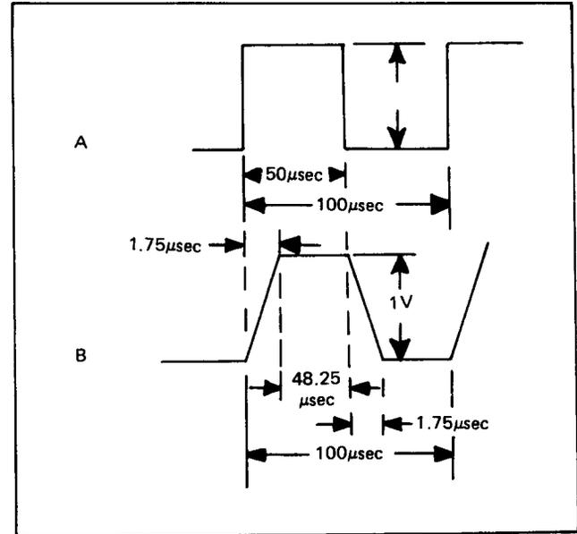
total slope periods equal to  $1.75 \mu\text{sec}$ . A comparison of the results will show the measurement error due to the finite bandwidth. Using Figure 2-6, Part B, for a reference, the total rms and dc levels are:
