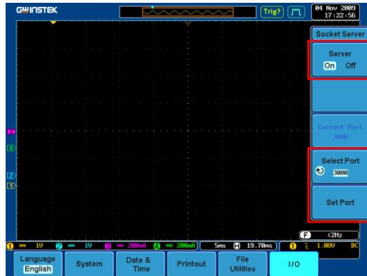
18. To check to see if the Ethernet settings are working enter the DSO's IP address into a browser: **172.16.1.3**
