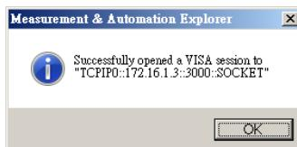
25. Press *OK*, and then press *Finish* on the New VISA TCP/IP Resource panel.
