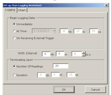
6. By default the measurements are plotted as a graph as soon as the data logging starts. Press the **Chart tab** to edit the chart behavior.
