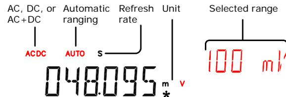
Manual ranging To select the measurement range manually, press the Up/Down keys.
